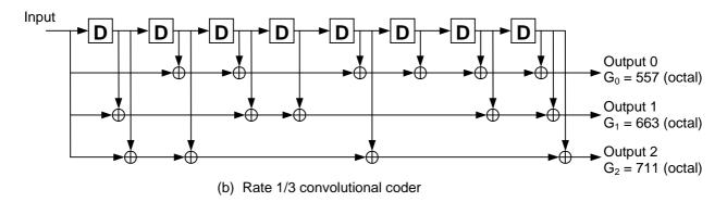
Figure 3: Rate 1/2 and rate 1/3 convolutional coders
